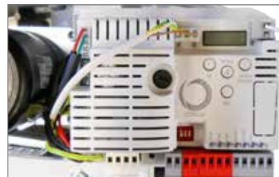
CT102 24 control board with integrated receiver
